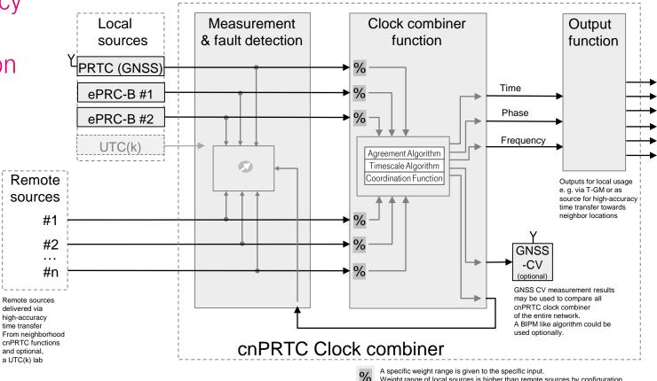
Weight range of local sources is higher than remote sources by configuration. Due to specific measurement results, weight can be automatically adjusted. In case of problems, the specific input can be squelched.
